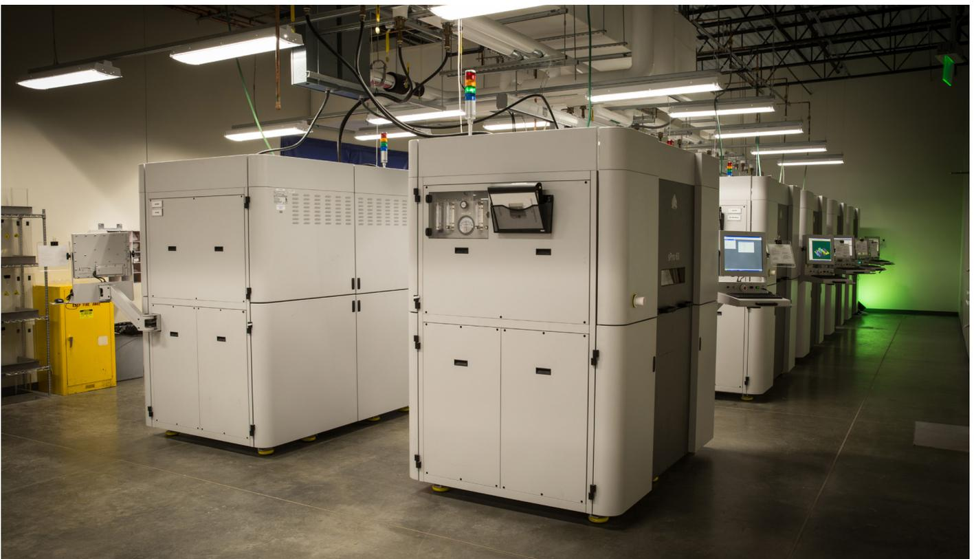
SLS printers at Protolabs' additive manufacturing facility in the U.S.
