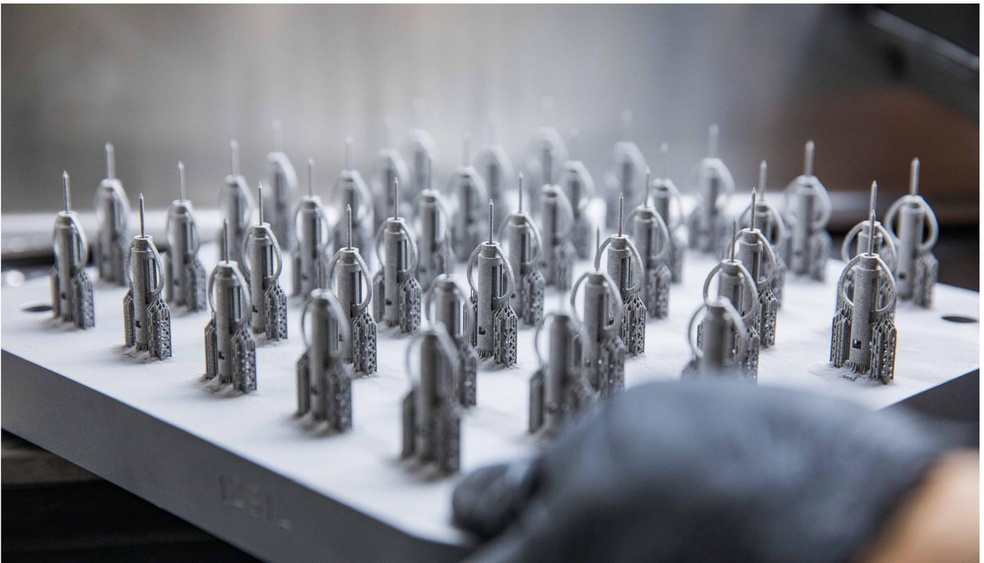
Direct metal laser sintering (DMLS) is capable of 3D printing complex and organic part geometries in a range of metal materials
